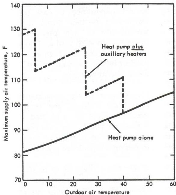
The solid line in Figure 1 shows the maximum supply air temperature leaving a typical 3 ton heat pump (1200 CFM flowing) as a function of outdoor temperature. Note that the values range from just over 80° F to about 105° F --- cold air, by furnace standards.
