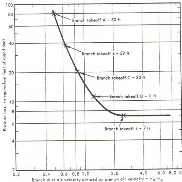
plenum ( $V_p$ ) just upstream of the fitting. This velocity ratio is really a measure of the momentum of the two (branch and plenum) moving air streams. What does the graph tell us?
