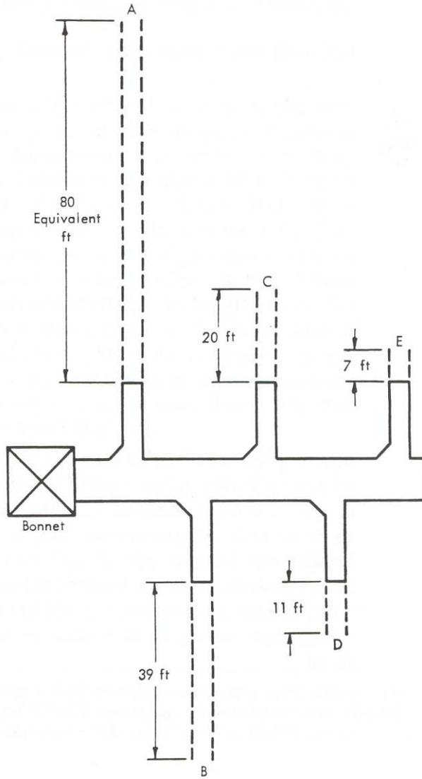
**Figure 3. EQUIVALENT LENGTH of take-off fittings when added to the actual duct length makes the closest branch the longest run in terms of resistance to air flow. Result: first branch delivers less air than last branch.**
