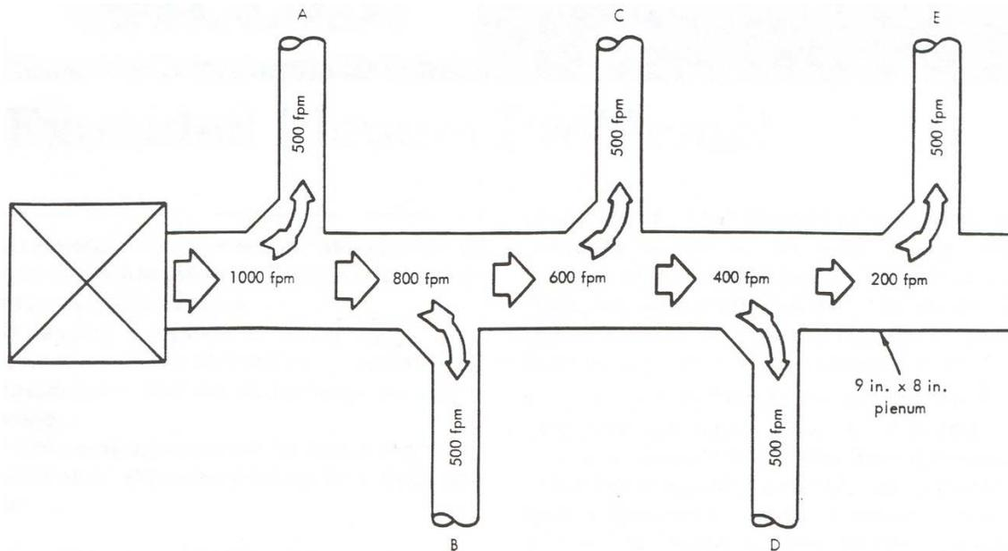
**Figure 2. An EXTENDED PLENUM. Unlike a reducing truck duct, is a constant size along its entire length. As air is diverted out succeeding branch runs, the velocity of the air remaining in the main decreases. Thus, the air initially has greater momentum and it can be harder to turn into a branch duct.**
