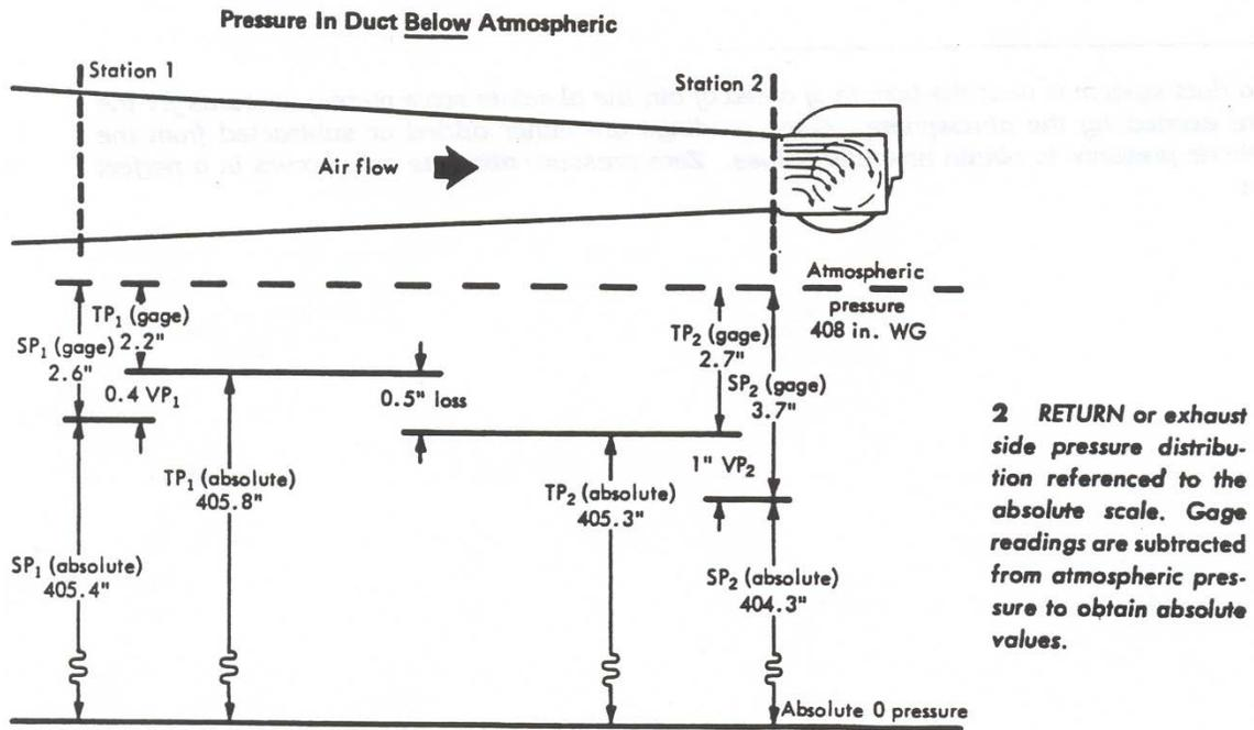
Thus, while numerically gauge **TP** readings are less than gauge **SP** measurements, and gauge **TP** readings increase in the direction of flow on the return side (from 2.2 to 32.7 in this example), reference to absolute values clearly resolves any paradoxes. **TP** (absolute) always decreases in the direction of flow and **TP** (absolute) always equals the sum of **VP** and **SP** (absolute) on either side of the fan.
